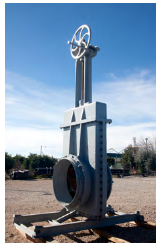
Restoration of a DN1000 gate valve
