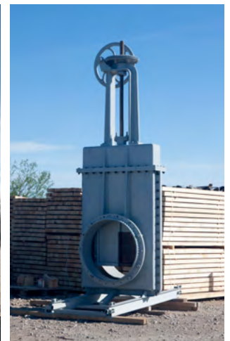
Restoration of a DN1000 gate valve
