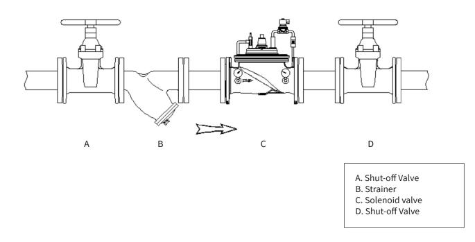
In order to carry out the setup and maintenance of a hydraulic valve, it is essential to install the following elements:
