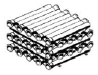
Bottom layer. Laying and wedging of the bottom layer is identical to the first method, but the pipes are sockets to spigos; their barrels are in contact. In addition, the sockets project beyond the spigots of adjacent pipes by the whole socket length, plus 5 dm. for Dn ≥ 150 pipes stacking is on
