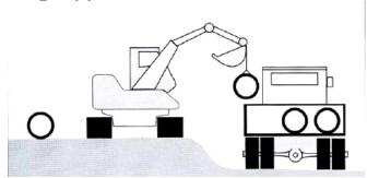
Unless specified otherwise, string the pipes out along the trench side opposite the excavated material, with the sockets pointing in the direction of laying (spigot end directed towards start of laying).
