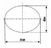
% OVALITY =  $\frac{DM - dm}{DM + dm} \times 100$
